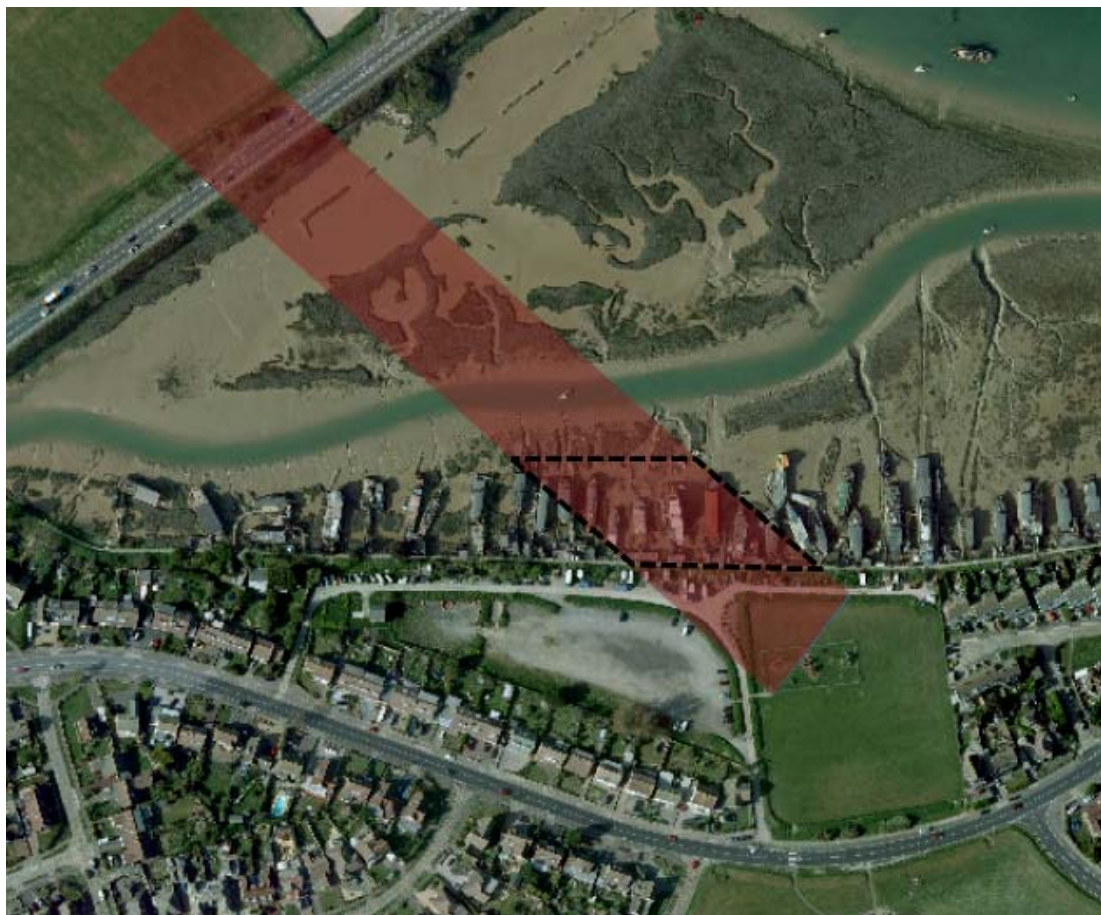
Figure 3: Potential landfall location south of Norfolk Bridge, showing indicative HDD corridor requirement (red)
